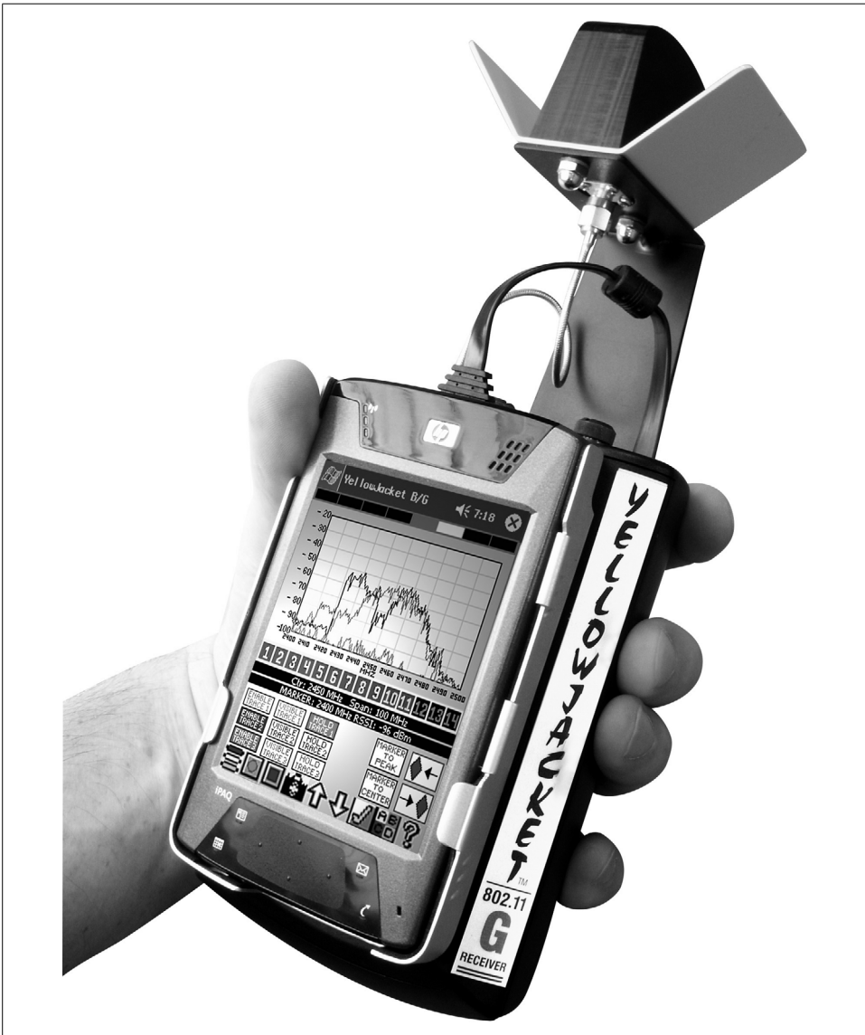
Figure 10-12. Wireless network maintenance tools, such as Yellowjacket, can guard against rogue access points
